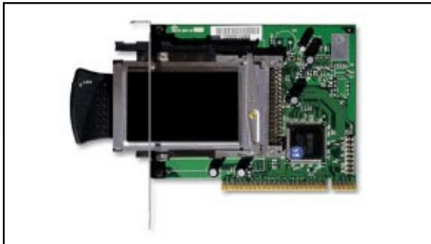
Wireless LAN PCI card (with a wireless LAN PCMCIA card in the slot.)
